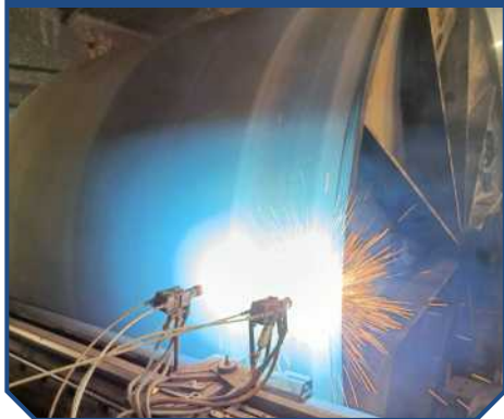
Pure Copper Coating by Flame Spray Process
